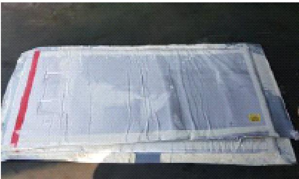
Fig. 2. Steps for obtaining reusable VIPs from end-of-life refrigerator.
